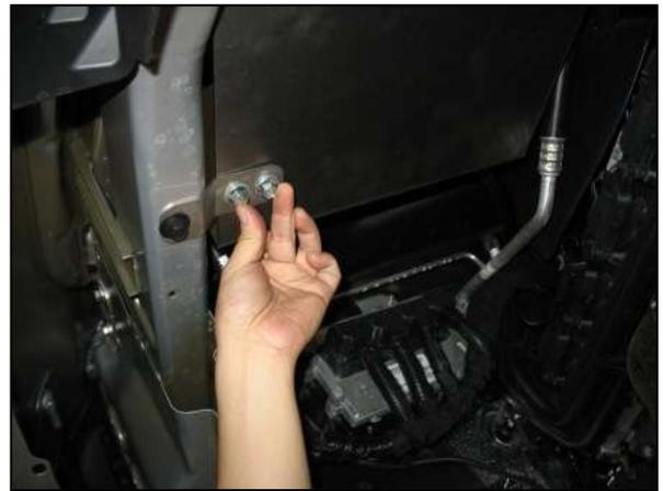
m. At the bottom bracket, hold 2 M8 bolts and 2 washers in position, aligning the bracket to the heat shield.
