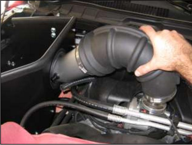
x. Install the intake pipe assembly, inserting the open end through the large hole in the heat shield while also mounting the elbow inlet onto the throttle body neck.
