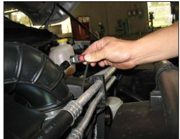
d. Unlock the intake air temperature (IAT) sensor connector by sliding the red tab and pressing the clip to disconnect the wiring harness from the sensor.
