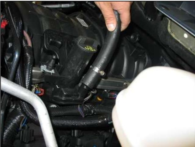
b. Install the 3/4" ID hose and 1 1/4" hose clamp as shown.
