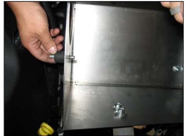
o. Install the rubber isolator mount on the outside of the heat shield assembly as shown.
