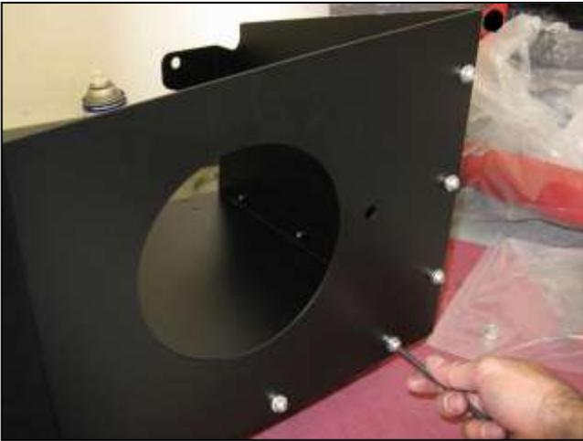
c. Now attach side Panel "B" to both panels "A" and "C" with 9 more M6 button head bolts, lock washers, and flat washers. Install the bolts loosely at first, then tighten them once the panels are in the correct position.
