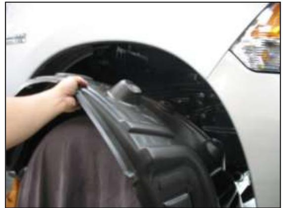
b. Remove the fender liner from the vehicle.
