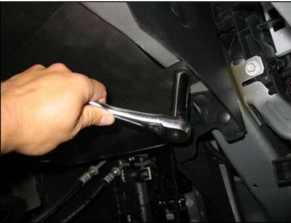
f. On the bottom side of the heat shield, secure the tab coming off the heat shield to the vehicle using the bolt removed in Step 2c. Tighten the bolt about  $\frac{3}{4}$  of the way into the thread for now.
