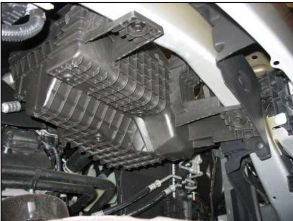
c. With the fender liner removed, access the air box from the bottom of the fender well and remove the 2 bolts securing the air box to the vehicle. Keep the bolts for use in a later step.
