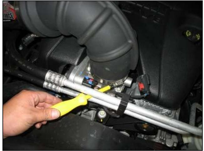
y. Tighten the smaller hose clamp of the elbow inlet at the throttle body.
