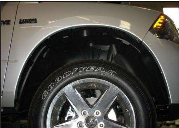
a. Remove all fasteners securing the passenger side fender liner. **WARNING:**After dropping the liner, be sure to unclip the ABS sensor wiring harness attached to the engine side of the liner.
