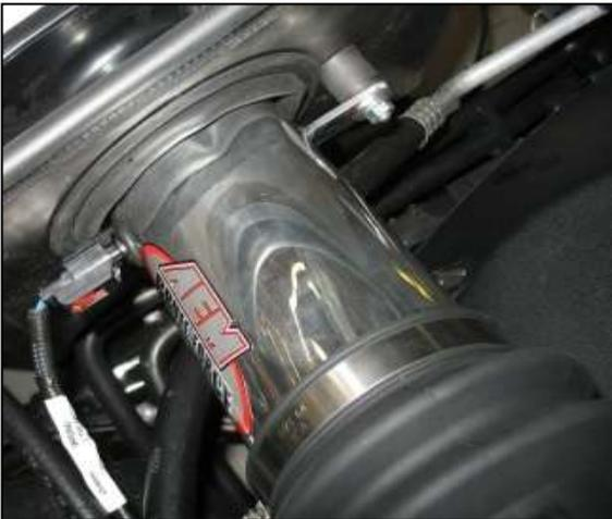
z. Connect the IAT sensor cable extension to the original wiring harness and lock the red tabs on the female connectors. Connect the opposite end of the IAT sensor cable extension to the IAT sensor.
