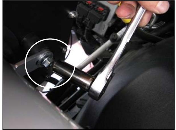
ac. Shift the inlet pipe until the slot in the mounting bracket lines up with the isolator bolt mounted on the heat shield. Place one 8mm flat washer and one M8 nut on the bolt and fully tighten. Now go back and fully tighten the larger air filter and inlet pipe hose clamps.
