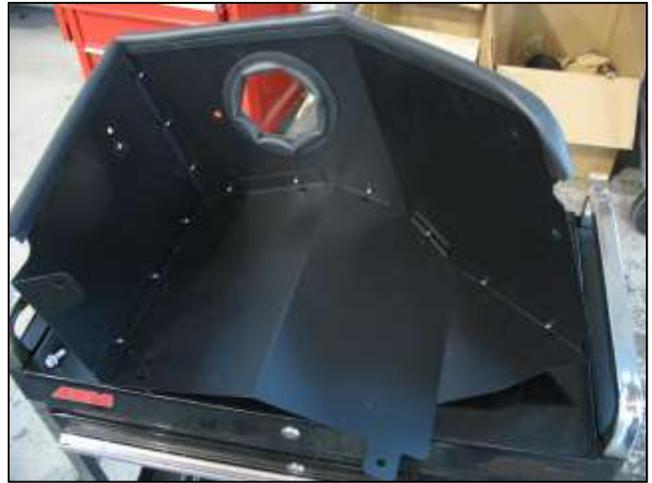
d. Here is the complete heat shield assembly. You may install the sponge rubber gaskets in the large hole (medium length gasket) and along the top edges (short and long gaskets) as shown at this time. Trim any excess as needed.
