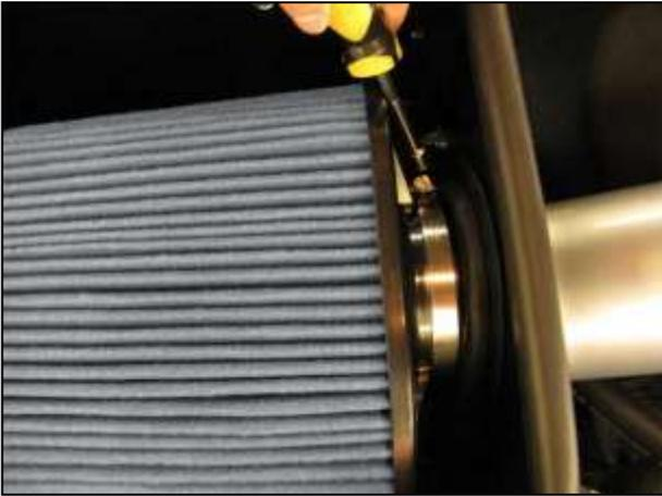
ab. Place the large hose clamp over the air filter's inlet. Place the air filter inside the heat shield and then fully seat the filter onto the filter adapter. Insert the open end of the inlet pipe and loosely secure the hose clamp to hold the air filter in place.
