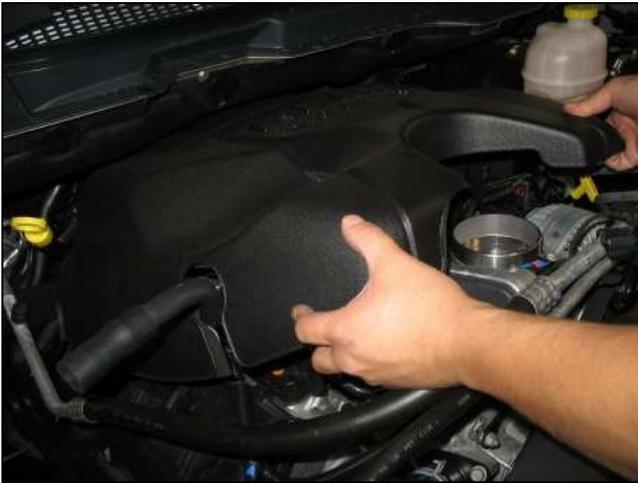
k. Remove the engine cover by lifting the front of the cover and then pulling forward.
