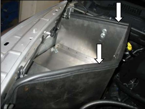
r. Install the short and the long sections of the rubber sponge edge gasket along the top edge of the heat shield as shown.
