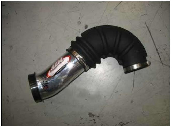
w. Install the inlet pipe into the adapter elbow, use soapy water to ease installation if necessary. Install the adapter insert into the open end of the inlet pipe.
