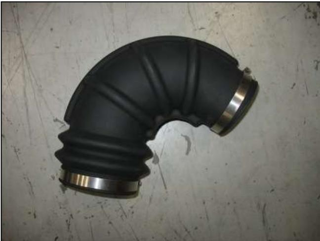
v. Loosely install hose clamps onto the intake adapter elbow as shown. Use hose clamp (9464) on the larger end and hose clamp (9452) on the smaller end.
