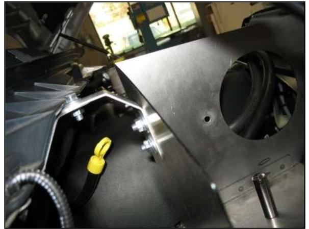
g. Install the rear bracket onto the top lip of the fire wall as shown. Use (Qty. 3) M8 x20mm bolts, (Qty. 3) nuts and (Qty. 6) washers to secure the bracket.
