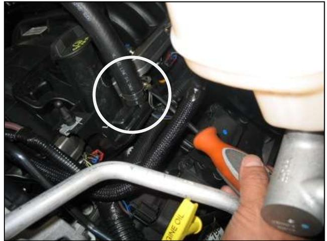
c. With the hose fully engaged on the nipple, fully tighten the hose clamp.
