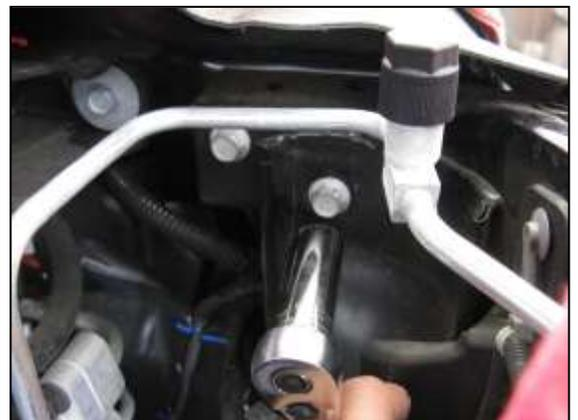
i. On the passenger side of the radiator support, remove the long bolt as shown.
