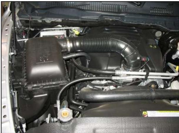
Factory air box system installed
