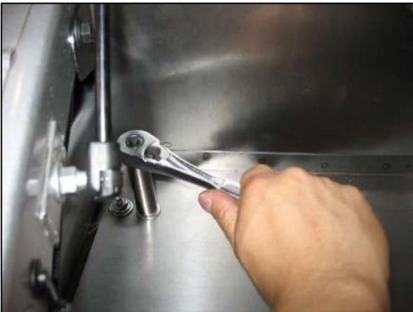
n. Install 2 M8 washers and 2 M8 nuts to secure the bolts positioned in the previous step. Now go back and tighten all the heat shield bracket nuts and bolts installed.
