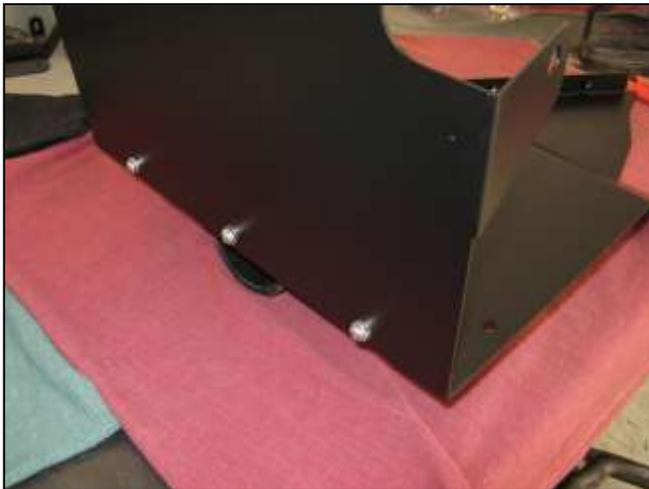
a. Attach the rear heat shield panel "C" to the bottom heat shield panel "A" using 3 of each of the following: M6 x 12mm button head bolts, 6mm lock washers, and 6mm flat washers. Leave the bolts loose for now.
