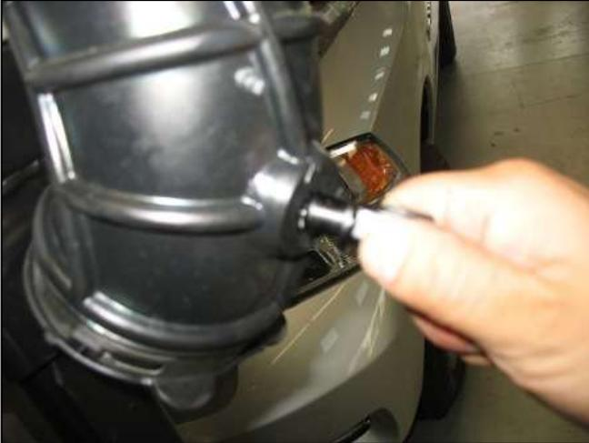
t. Carefully remove the inlet air temperature (IAT) sensor from the OEM inlet duct.
