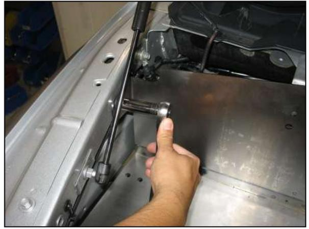
e. Carefully position the heat shield into the vehicle. Use the bolt removed in Step 2i to hold the heat shield in place. Tighten the bolt about  $\frac{3}{4}$  of the way into the thread for now.
