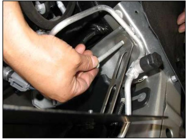
k. Secure the front tab of the bracket to the vehicle using the long bolt removed in step 4i.
